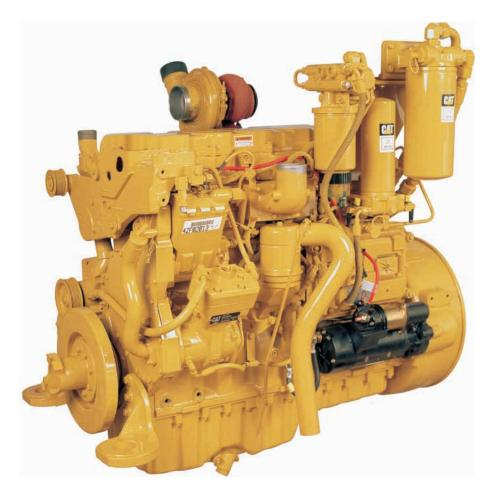
**Cat C-9 ETA Engine.** The innovative Cat C-9 diesel engine delivers largeengine performance from a compact engine design. This six-cylinder engine is turbocharged and air-to-air aftercooled. With high displacement and low rated speed, the C-9 provides excellent fuel economy and durability that can significantly reduce operating costs.
